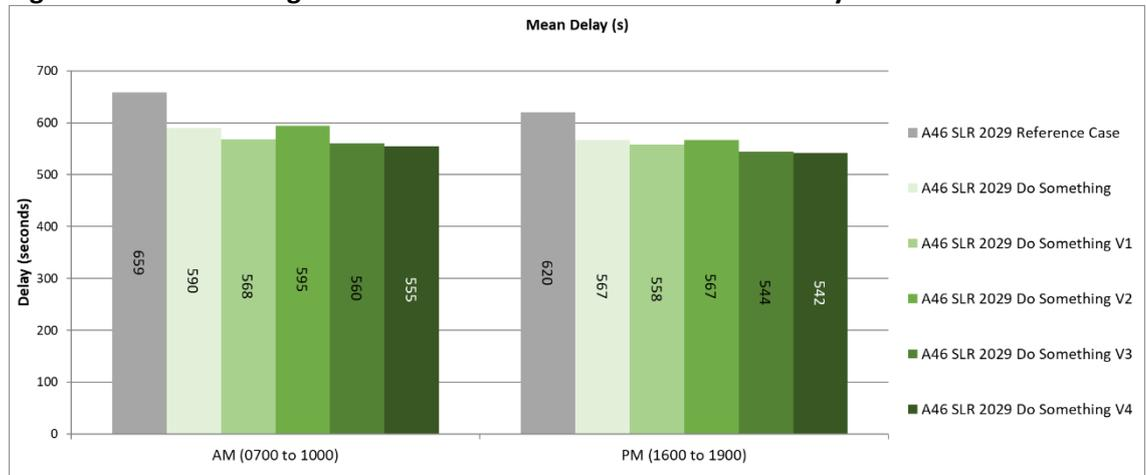
5.35 The network wide delay statistics presented within **Figure 25** demonstrate substantial reductions in journey times across the network, during the AM and PM periods, in each of the Do Something scenarios assessed. The AM reductions are at or below the levels observed within the Do Minimum testing whilst, in the PM, the reductions are significantly greater than those observed within the Do Minimum testing.
