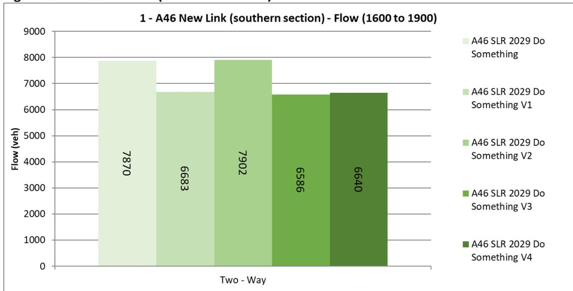
5.41 The link flows presented for the southern section of the A46 link across the AM and PM period demonstrate that the Do Something V2 scenario results in the highest two way traffic flows on the link itself. These results suggests that the complete closure of Gibbet Hill Road to through trips has the most noticeable impact in terms of drawing trips onto the new link road.
