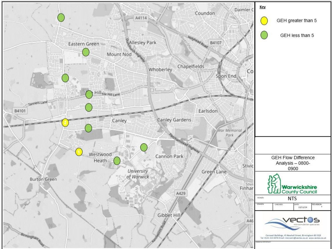
**Figure 55 Flow Difference Analysis (GEH) – PM Peak Hour**
