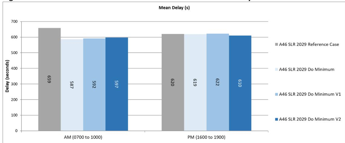
5.19 **Figure 19** illustrates the impact on network wide delay in each of the Do Minimum scenarios tested, compared with the 2029 Reference Case. The results indicate that the inclusion of the partial link improves average journey times during the AM period, however, the PM period results suggest that the inclusion of the partial link does not deliver any changes to the network wide performance of the model.
