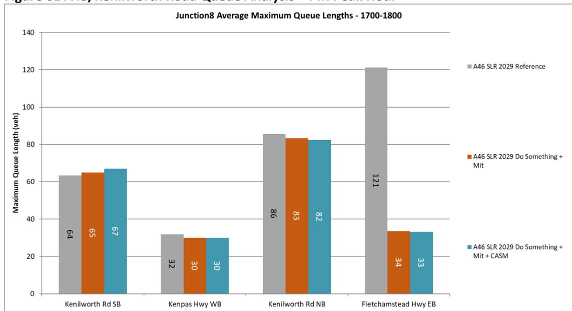
7.18 The queue analysis graphs presented within **Figure 60** and **Figure 61** demonstrate that across the AM and PM period there are no notable changes in queue lengths across the junction as a result of factoring into the modelling the reassignment effects.
