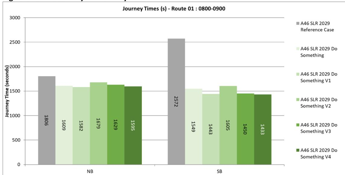
5.46 The AM peak hour journey times on the A45 are presented within **Figure 32**. As with the Do Minimum scenario analysis, the inclusion of the link results in significantly reduced journey times on the A45 southbound in each of the Do Something scenarios when compared with 2029 Reference Case conditions and that these reductions are also significantly greater than any reductions achieved through the implementation of the options identified within the Do Minimum testing
