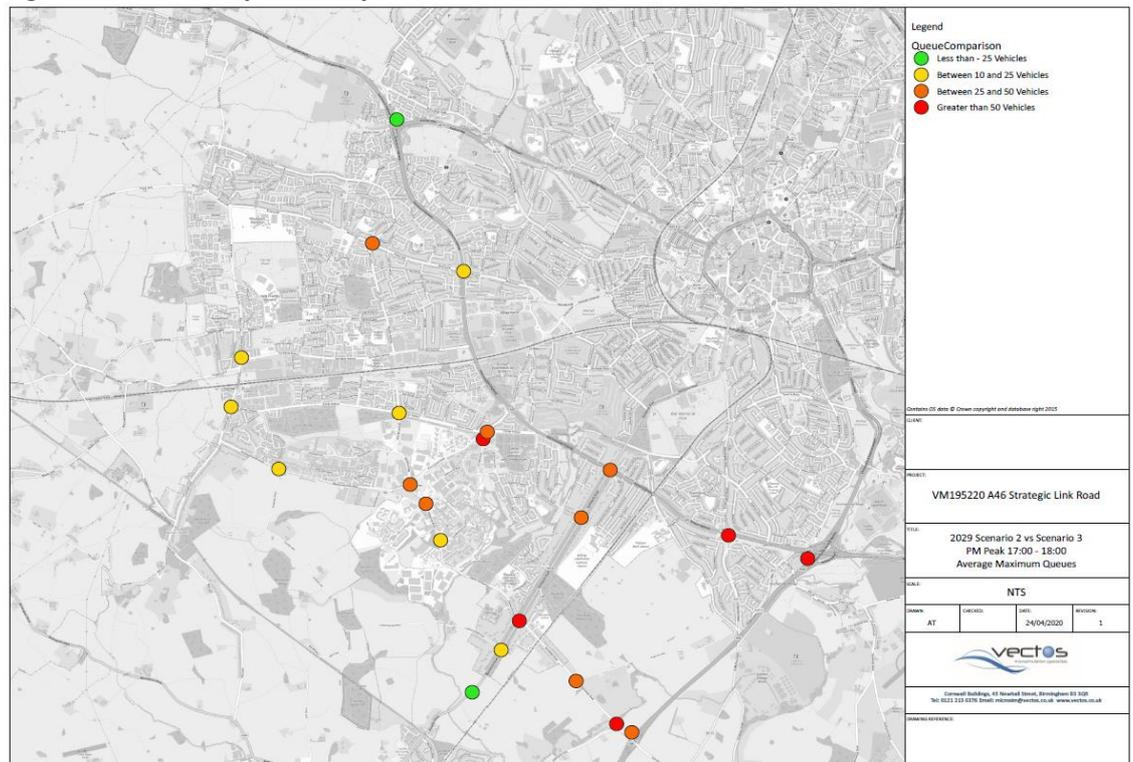
7.39 The analysis presented within **Figure 66** and **Figure 67** illustrates the queue impact between the 2029 Reference and 2029 Do Something + Mitigation + Growth scenarios. In line with the network wide statistics results presented, this analysis suggests that the network is
