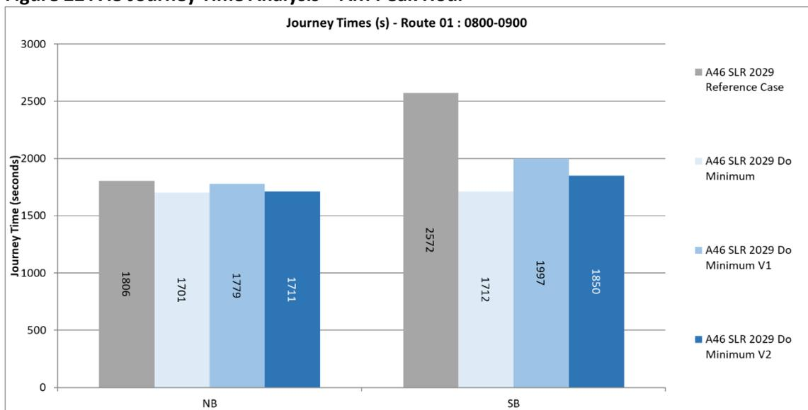
5.26 **Figure 22** presents the impact on journey times on the A45 in the AM peak hour, in each of the Do Minimum scenarios. The results demonstrate that the introduction of the partial link between the A46 and A429 has the potential to reduce southbound journey times during the AM peak.
