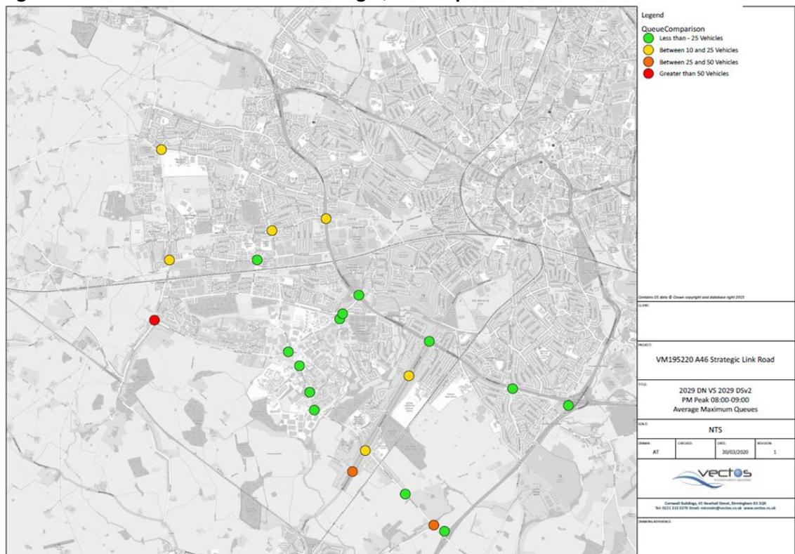
6.11 The AM peak hour queue length analysis, presented within **Figure 37**, reveals that the Do Something scenario results in significant number of queue length reductions across the network when compared with 2029 Reference Case conditions, notably along the A45 and Gibbet Hill Road.
