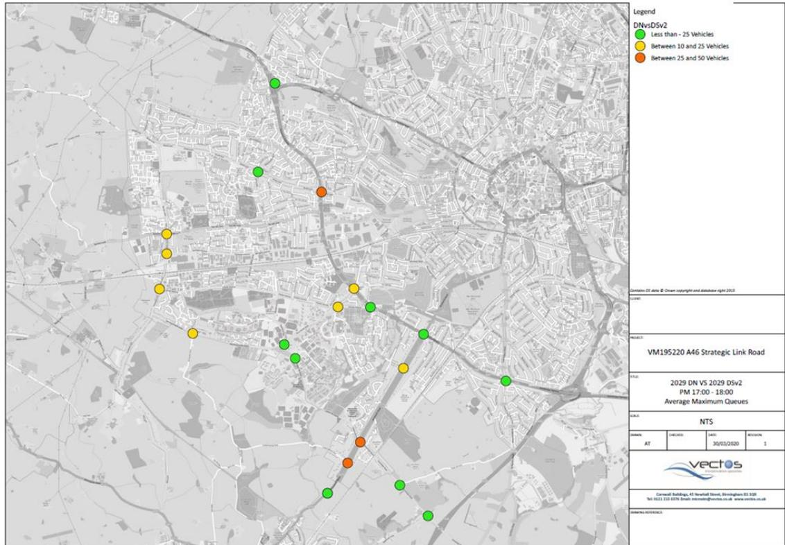
6.13 The PM peak hour queue length analysis, presented within **Figure 38**, reports a similar pattern to the AM results, with a significant number of junctions at which queue lengths reduce, notably along the A45 and Gibbet Hill Road.
