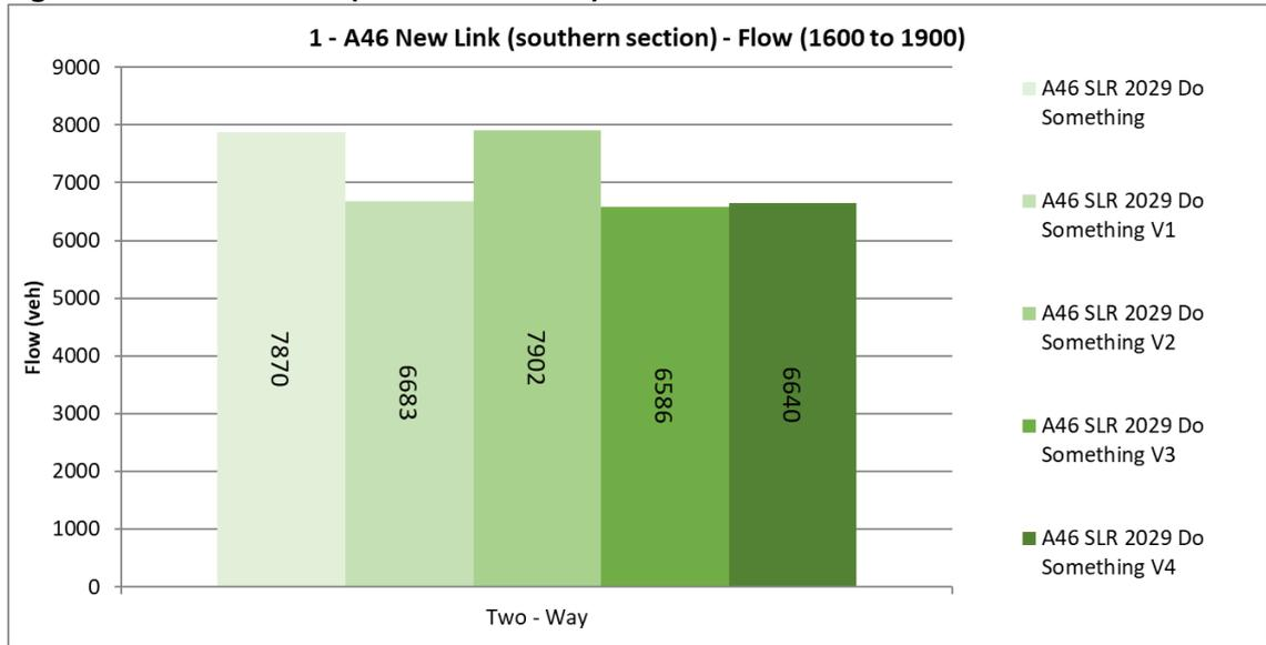
5.41 The link flows presented for the southern section of the A46 link across the AM and PM period demonstrate that the Do Something V2 scenario results in the highest two way traffic flows on the link itself. These results suggests that the complete closure of Gibbet Hill Road to through trips has the most noticeable impact in terms of drawing trips onto the new link road.
