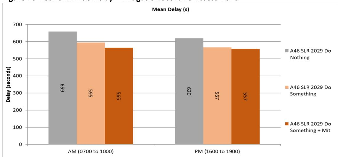
6.30 **Figure 46** demonstrates the impact on network wide delay once the mitigation identified is included within the network. The AM period results suggest that average journey times are reduced by a further 30 seconds over the Do Something scenario, once the mitigation is included.
