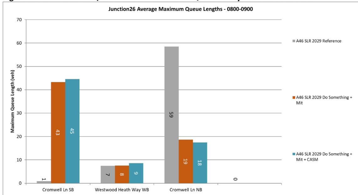
7.20 In a similar pattern to the analysis of the A45/Kenilworth Road junction, the queue results during the AM peak hour presented within **Figure 62** demonstrates no change when comparing the scenarios with and without the reassignment effects included.
